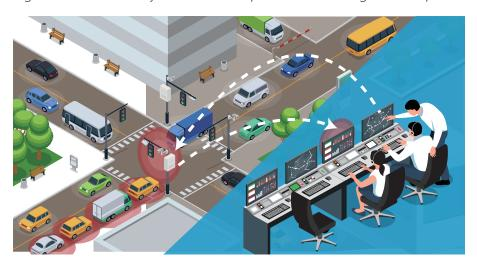
This system is designed to monitor traffic conditions through various traffic data which are from Vehicle Detectors (VD) and eTags, to adjust traffic signals in real-time. Furthermore, it also provides guidance for alternative routes, reduces traffic congestion, increases traffic speed, and shortens travel time.
